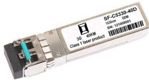
The optical output can be disabled by a TTL logic high-level input of Tx Disable, and the system also can disable the module via I2C. Tx Fault is provided to indicate that degradation of the laser. Loss of signal (LOS) output is provided to indicate the loss of an input optical signal of receiver or the link status with partner. The system can also get the LOS (or Link)/Disable/Fault information via I2C register access.
